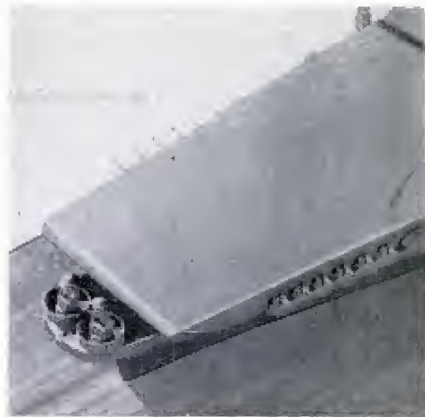
Closeup views at the bow. In the left-hand photo the flight-deck assembly has been removed to expose the deck fittings on the forecastle. Note in the right-hand photo the batteries of 20-mm. AA guns, each side
